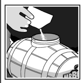
1.1 Fill keg with lukewarm water to the 4-quart mark on the back. Add ½ pack of the No-Rinse cleanser and stir until dissolved. Once dissolved, the sanitizing solution is ready to use. Screw on lid and swirl so that the solution makes contact with all parts of the keg, including the lid.
